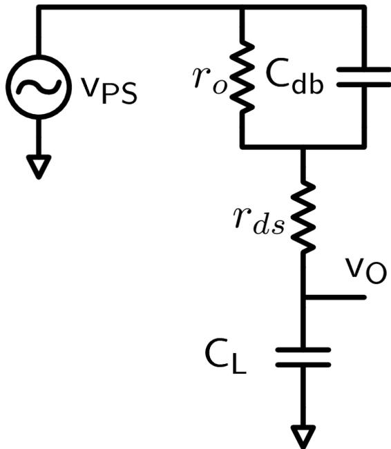
$$\frac{V_O(s)}{V_{PS}(s)} \approx \frac{sr_o C_{db} + 1}{(sr_o C_L + 1)(sr_{ds} C_{db} + 1)}$$
