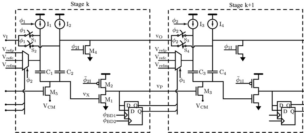
Fig. 7. Two stages of the 1.5 bit/stage zero-crossing-based pipelined ADC.
