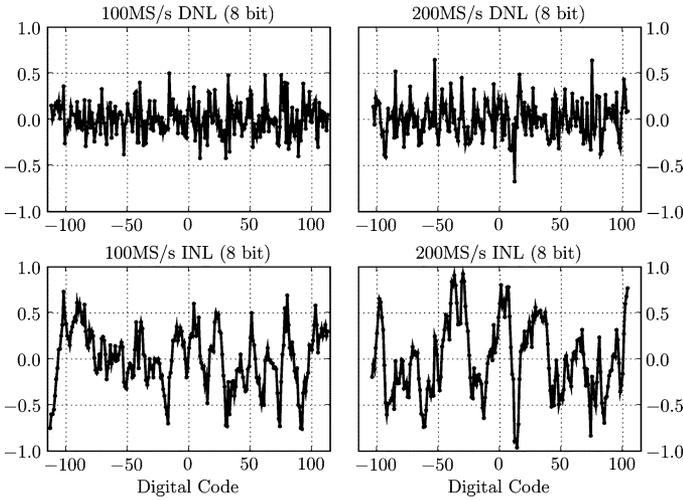
Fig. 13. DNL and INL plots for 100 MS/s and 200 MS/s operation.
