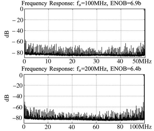
Fig. 14. Measure frequency response to near Nyquist rate input tone.
