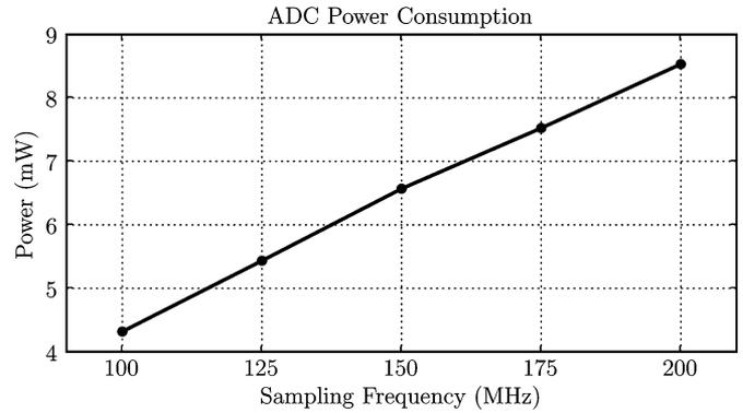
Fig. 15. Measured power consumption versus sampling frequency.
