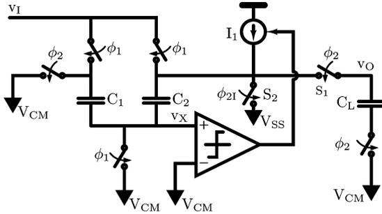
Fig. 2. Comparator-based switched-capacitor (CBSC) gain stage.
