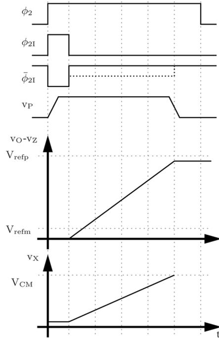
Fig. 6. Sample transient response of a ZCBC switched-capacitor gain stage.
