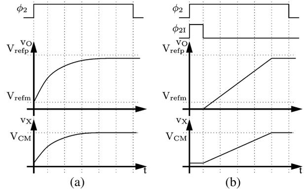
Fig. 3. Sample transient response of (a) an opamp-based and (b) a CBSC switched-capacitor gain stage.
