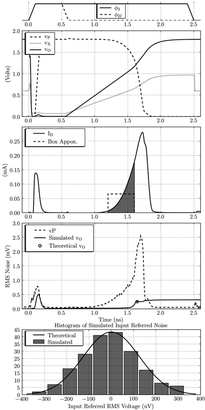
Fig. 16. Simulated transient response used for noise analysis verification.
