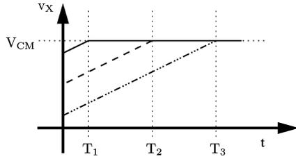
Fig. 4. Sample input waveforms into a CBSC comparator.
