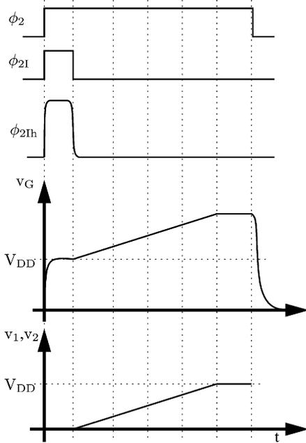
Fig. 9. Shorting switch timing diagram.
