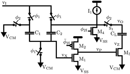
Fig. 5. Zero-crossing-based switched-capacitor gain stage.
