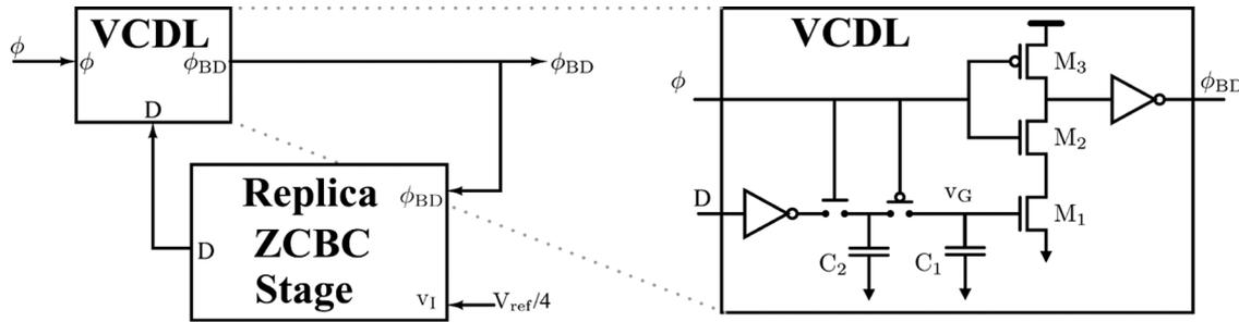
Fig. 11. The bit decision flip-flop phase generation circuit, including the voltage-control delay line implementation.
