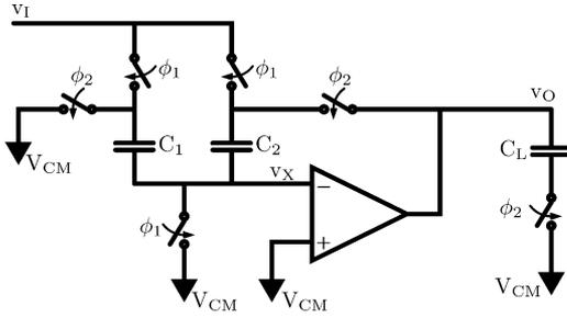
Fig. 1. Typical opamp-based switched-capacitor gain stage.
